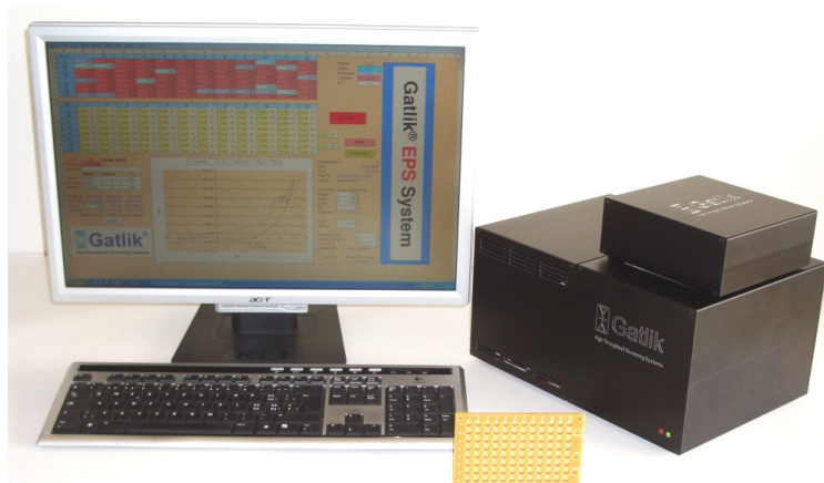
Figure 1. Gatlik® EPS System with Sensor-Plate-96.2TV3 and controlling & processing software.
