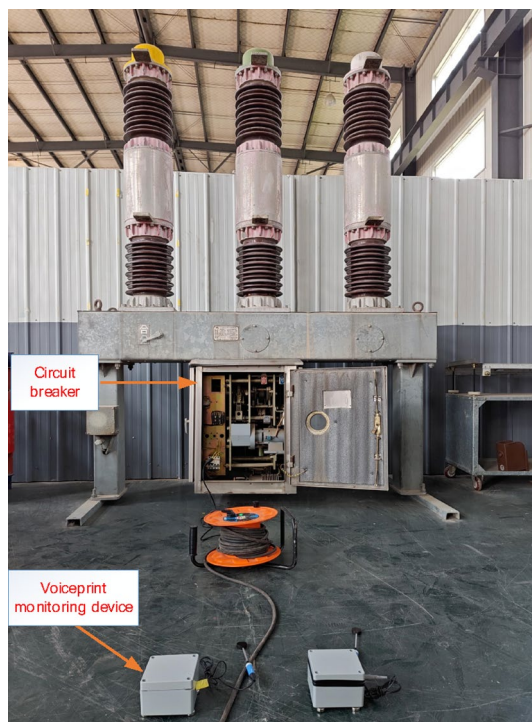
Figure 9. Voice print information monitoring test system.
