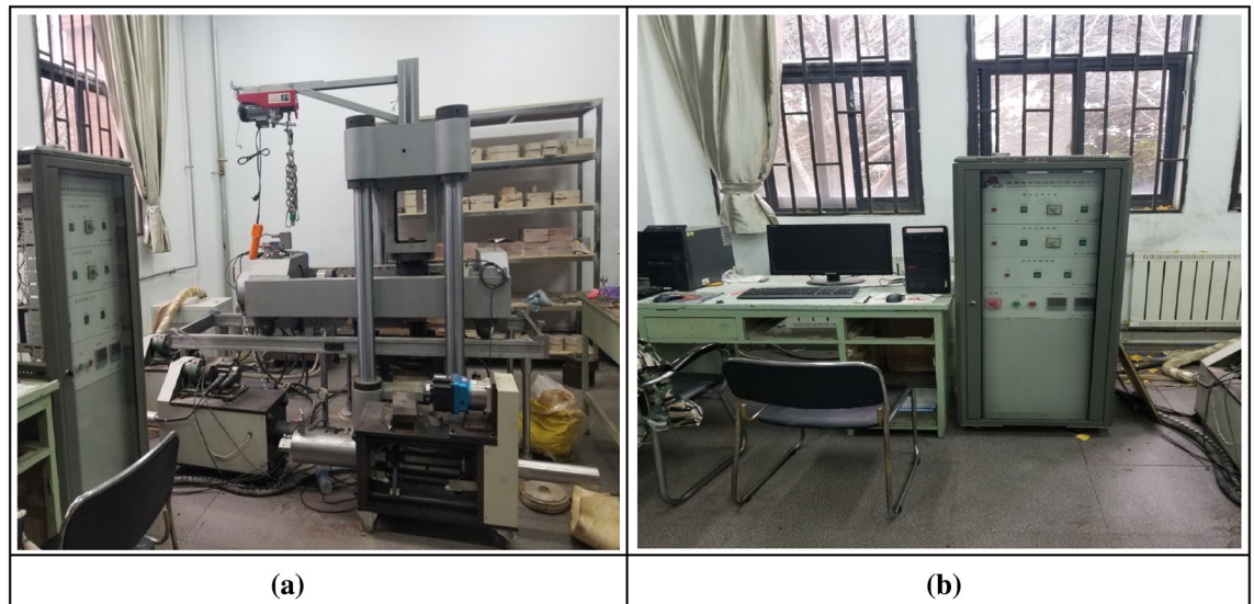
Figure 5. Shear seepage testing machine. (a) Straight shear testing machine. (b) Servo test system.
