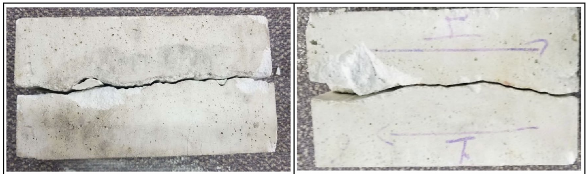
Figure 10. Side damage of jointed rock mass.
