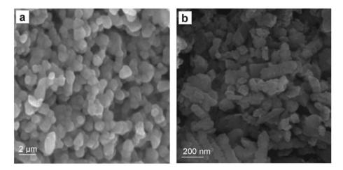
Figure 4. SEM microscopy of ZnO NPs (a) and H<sub>2</sub>O<sub>2</sub>/ZnO NPs composite (b).
