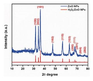
Figure 7. XRD pattern of ZnO NPs, and  $H_2O_2/ZnO$  NPs composite.
