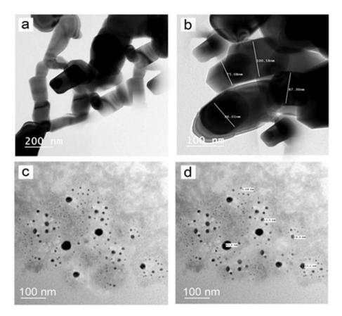
**Figure 5.** Transmission electron microscopy of ZnO NPs (**a**-**b**) clarified the hexagonal shape of zin oxide nanoparticles (**a**) and the diameter of NPs was ranged between 75.08 to 100.58 nm (**b**). Moreover,  $H_2O_2/ZnO$  NPs Micrographs exhibited the alteration in NPs shape to pentagonal (**c**) and the size of NPs in diameter was ranged from 5.48 to 34.6 nm (**d**).
