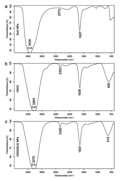
**Figure 6.** FTIR spectra of ZnO NPs (**a**),  $H_2O_2$  (**b**), and  $H_2O_2/ZnO$  NPs composite (**c**).
