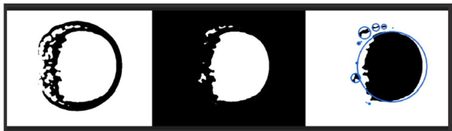
Figure 8. Image generated by the seed detection algorithm applied to the preprocessed image. The blue circles represent the detected objects, while the black regions correspond to the background. The top left panel shows the outlines of the objects, the top right panel shows the region where the flood-fill operation was applied to find the objects, and the bottom panel shows the detected objects with a circle around each one.
