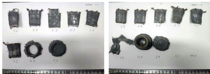
(a) A fragments of 48mm stun grenades (b) B fragments of 48mm stun grenades
