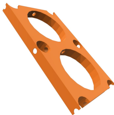
Figure 18. Interconnected cavities concept in the perforated layer (middle layer) of MarZ-6.
