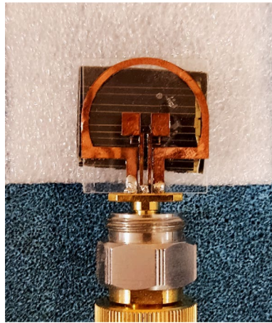
Figure 29. Antenna manufactured with a transparent substrate and placing a solar cell along with a 50Ω coaxial SAM port.
